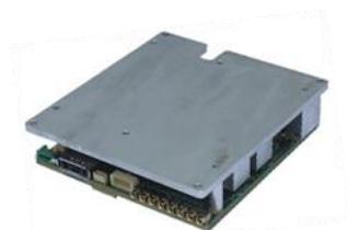
CHARM-100 with attached heat spreader
