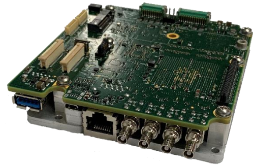
CHARM-100NX with attached heat spreader
